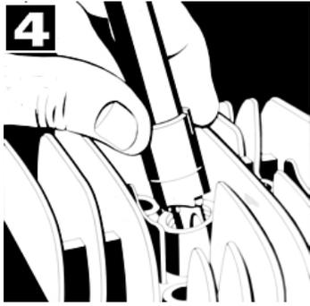
4. Using the wrench provided rotate the seat cutter. After a few turns lift the seat cutter to inspect the seat. Repeat operation until the seat is completely cleaned up. Remove the step tap from the hole.
