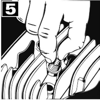
5. Make sure the hole is clean and dry. Lubricate the driver tool with Time-Sert driver oil. Screw the insert onto the prepared hole.
