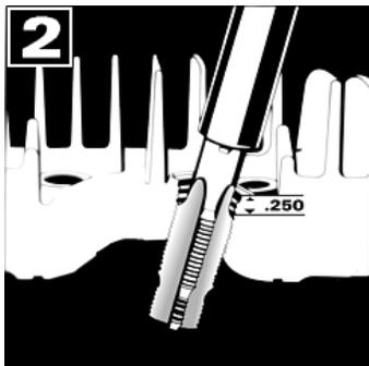
2. Using the wrench provided place wrench over tap and tap new threads. Continue to tap through until the cutting edges are approximately 1/4 inch below surface.
