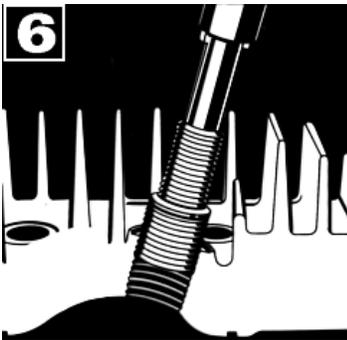
6. *Note: Tapered Seat inserts these inserts are silver plated and require sealer p/n 6020 on the outside of the insert.*
