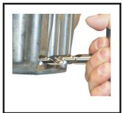
Use of a cutting fluid is recommended for drilling counterboring and tapping.
