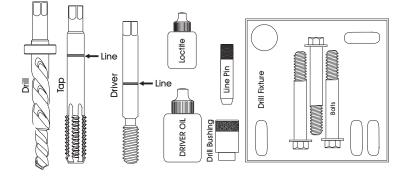
Tools: Step drill Tap Insert driver Bolts (3) Drill fixture Alignment pin Drill bushing Inserts (Qty 10) loctite Driver oil
