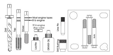
Tools needed: Drill fixture Drill bushing Alignment pin Bolts (3) Step drill Tap Insert driver B16 Spacer Inserts (Qty 10) loctite Driver oil
