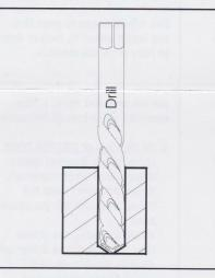
1. DRILL out old threads keeping drill square to surface of hole.
