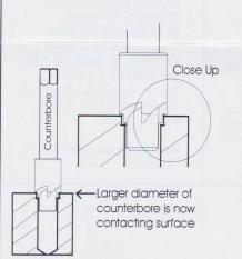
2. COUNTERBORE the hole to the full depth permitted by the tool. The counterbore tool has 4 cutting teeth and a larger diameter that is the stop.
